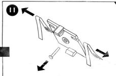
Remove the worn braids and guide pin from the braid plate.
