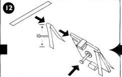
Fit new guide pin and braids to the braid plate. The braids should be folded so that the ends on top of the guide plate are 10mm long.
