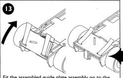
Fit the assembled guide plate assembly on to the chassis by engaging the front clip first and then the
