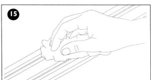
Always keep track clean by wiping over with a non-fluffy cloth, especially before putting the set away. Keep the pick-up rails shiny by rubbing carefully with a nylon "Scotch" washing-up pad or track cleaning rubber, reference R8087, obtainable from Hornby stockists.
