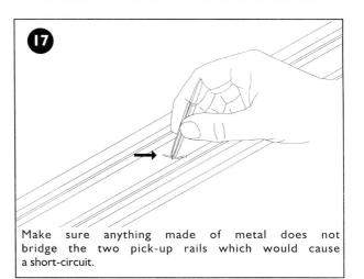
If a short-circuit does occur, the automatic cut-out in the transformer will come into operation and shut off power to the track. In this case, unplug the transformer from the wall socket, eliminate the reason for the short-circuit and plug the transformer back in again. Note: The transformer must remain unplugged for at least 45 seconds to allow the cut-out to reset itself.
