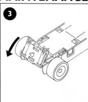
Turn the chassis over and remove the braid plate from its front clip.
