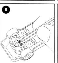
Remove any carpet fibres, pet hairs etc., from around the car's axles and gear wheel.
