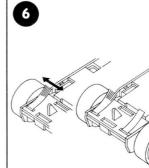
Refit the car body and tease out the ends of the braids so they make good contact with the pickup rails in the track.
