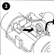
Carefully bend the orange/brown capacitor back to reveal the guide blade clip. Unclip the rear of the guide blade by pressing BACK & DOWN on the clip from the inside of the chassis with a SCREWDRIVER.
