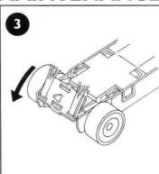
Turn the chassis over and remove the braid plate from its front clip.
