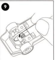
Periodically, oil the axle bearings and gear wheel with one drop of light machine oil.
