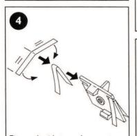
Fit new braids to replacement guide plate. The braids should be folded so that the ends on top of the guide plate are 10mm long.
