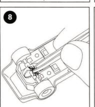
Remove any carpet fibres, pet hairs etc., from around the car's axles and gear wheel.
