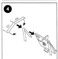
Fit new braids to replacement guide plate. The braids should be folded so that the ends on top of the guide plate are 10mm long.
