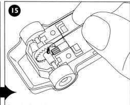
Periodically, oil the axle bearings and gear wheel with one drop of light machine oil.
