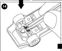
Remove any carpet fibres, pet hairs etc., from around the car's axles and gear wheel.
