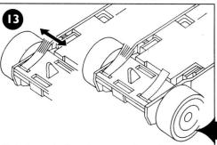
Refit the car body and tease out the ends of the braids so they make good contact with the pick-up rails in the track.
