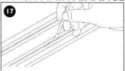
Keep the slot between the pick-up rails free from anything which would prevent the guide fin from travelling along it freely.
