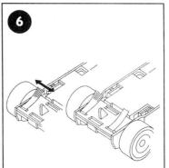
Refit the car body and tease out the ends of the braids so they make good contact with the pickup rails in the track.
