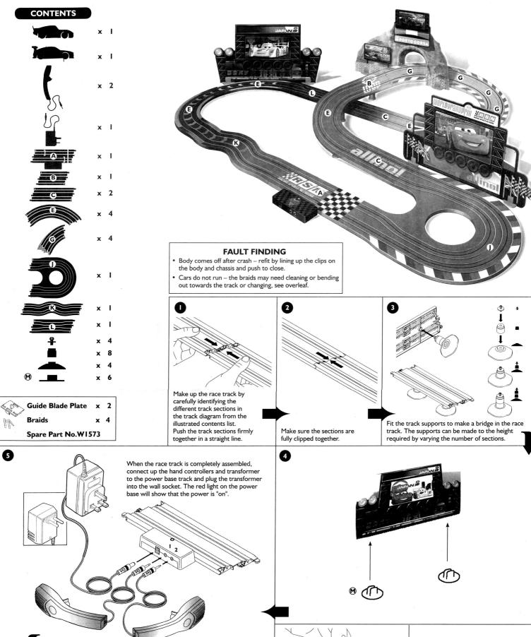
Place a car on one side of the track with its guide fin in the slot between the metal rails. Slowly squeeze the trigger of its hand controller to make the car go around the track. Now put the other car on the other lane and use the other controller to test it. If both cars work on both lanes of the track, you are ready to race. Remember – the more you squeeze the trigger, the faster the cars will go, so take it easy at first!
