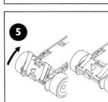
Fit the assembled guide plate assembly on to the chassis by engaging the front clip first and then the rear clip.
