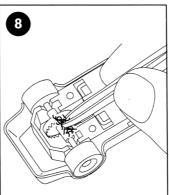
Remove any carpet fibres, pet hairs etc., from around the car's axles and gear wheel.
