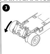
Turn the chassis over and remove the braid plate from its front clip.
