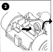
Carefully bend the orange/brown capacitor back to reveal the guide blade clip. Unclip the rear of the guide blade by pressing BACK & DOWN on the clip from the inside of the chassis with a SCREWDRIVER.
