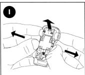
After a while, the pick-up braids underneath the cars may become worn out and need replacing. To do this, turn the car over and unclip the body from the chassis.
