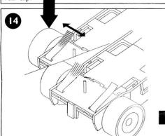
Refit the car body and tease out the ends of the braids so they make good contact with the pick-up rails in the track.
