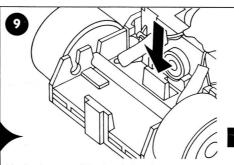
Unclip the rear of the braid plate by pressing down on the clip, from insidethe car, as shown in the diagram. You may have to use a
