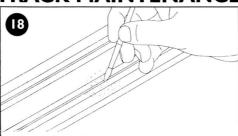
Keep the slot between the pick-up rails free from anything which would prevent the guide pin from travelling along it freely.
