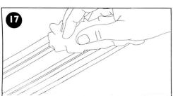
Always keep track clean by wiping over with a non-fluffy cloth, especially before putting the set away. Keep the pick-up rails shiny by rubbing carefully with a nylon "Scotch" washing-up pad or track cleaning rubber, reference R8087, obtainable from Hornby stockists.
