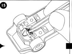
Remove any carpet fibres, pet hairs etc., from around the car's axles and gear wheel.
