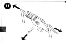
Remove the worn braids and guide pin from the braid plate.
