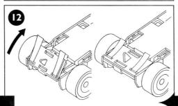
Fit the assembled guide plate assembly on to the chassis by engaging the front clip first and then the rear clip.
