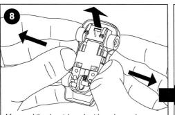
After a while, the pick-up braids underneath the cars may become worn out and need replacing. To do this, turn the car over and unclip the body from the chassis.
