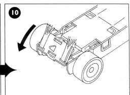
Turn the chassis over and remove the guide plate from its front clip.
