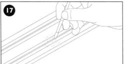
Keep the slot between the pick-up rails free from anything which would prevent the guide fin from travelling along it freely.
