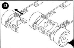
Refit the car body and tease out the ends of the braids so they make good contact with the pick-up rails in the track.
