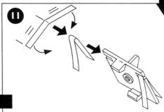
Fit new braids to replacement guide plate. The braids should be folded so that the ends on top of the guide plate are 10mm long.
