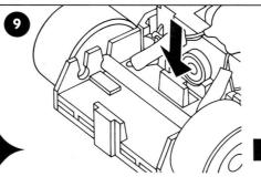
Unclip the rear of the guide plate by pressing down on the clip, from inside the car, as shown in the diagram. You may have to use a screwdriver to do this.
