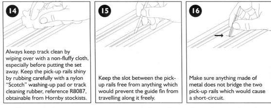
If a short-circuit does occur, the automatic cut-out in the transformer will come into operation and shut off power to the track. In this case, unplug the transformer from the wall socket, eliminate the reason for the short-circuit and plug the transformer back in again. Note: The transformer must remain unplugged for at least 45 seconds to allow the cut-out to reset itself.
